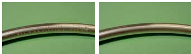
Figure 1: Blisters seen on a standard silver plated seal after 1,000 hours in air at 500°F
